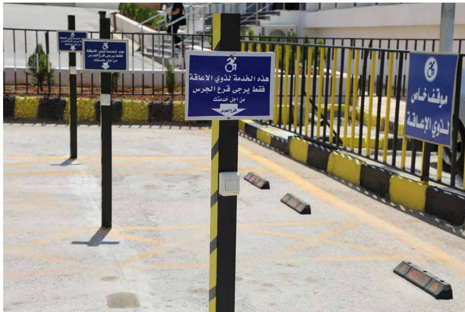
Designated parking spaces for vehicles of persons with disabilities, equipped with an alert bell in case of difficulty exiting the vehicle.
